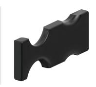
The PolyVee tensioning device enables easy tensioning of 2-rib and 3-rib PolyVee belts and is intended for roller pitches 75 mm and 100 mm. The tensioning device is designed for rollers and RollerDrive with a diameter of 50 mm. It cannot be used for tubes with tube sleeves or tapered elements.
